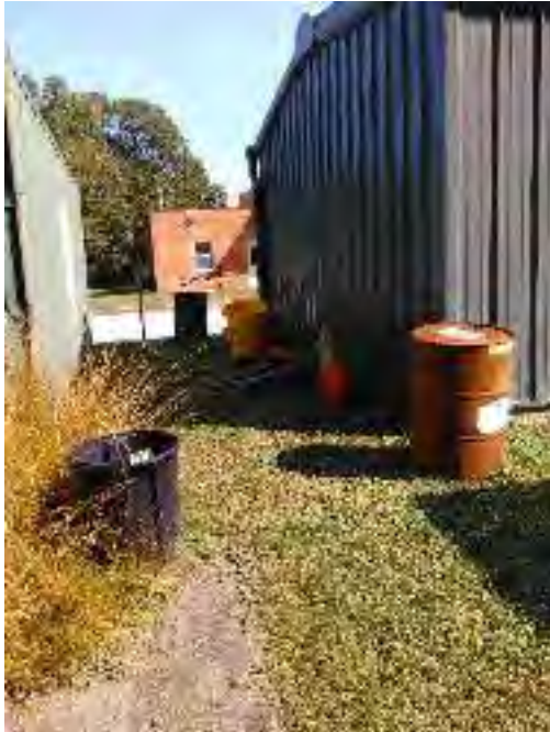
Figure 6: Improper liquid storage of drums.
