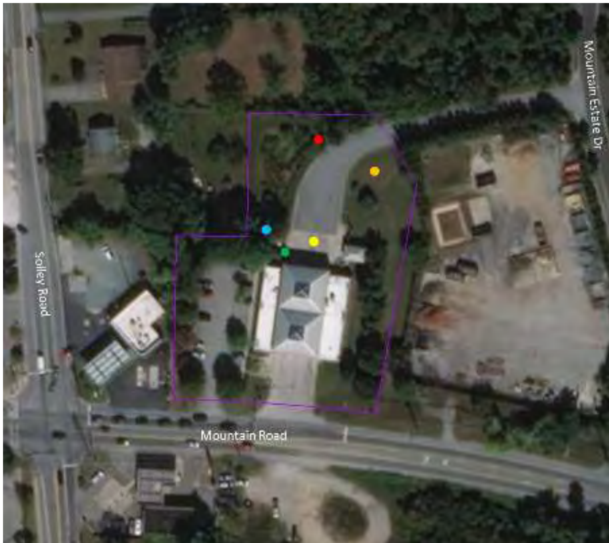
Figure 1: Aerial map of Armiger Fire Station Blue Circle = Parking lot outfall Red Circle = Unverified outfall from headwall, and rear drive inlets Orange Circle = Headwall inlet from grass conveyance channel Yellow Circle = Suspected washing station Green Circle = Dumpster and recycling area
