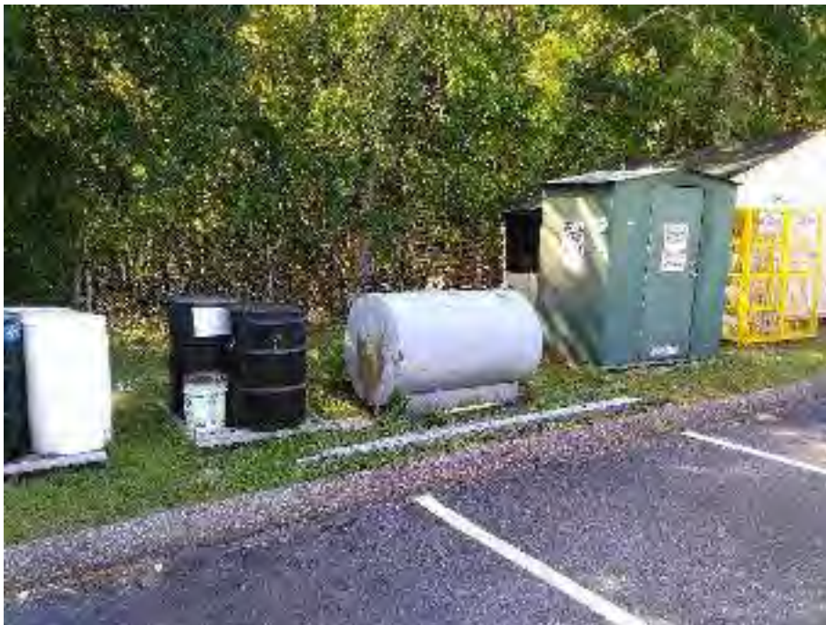
Figure 7: Improper liquid storage.
