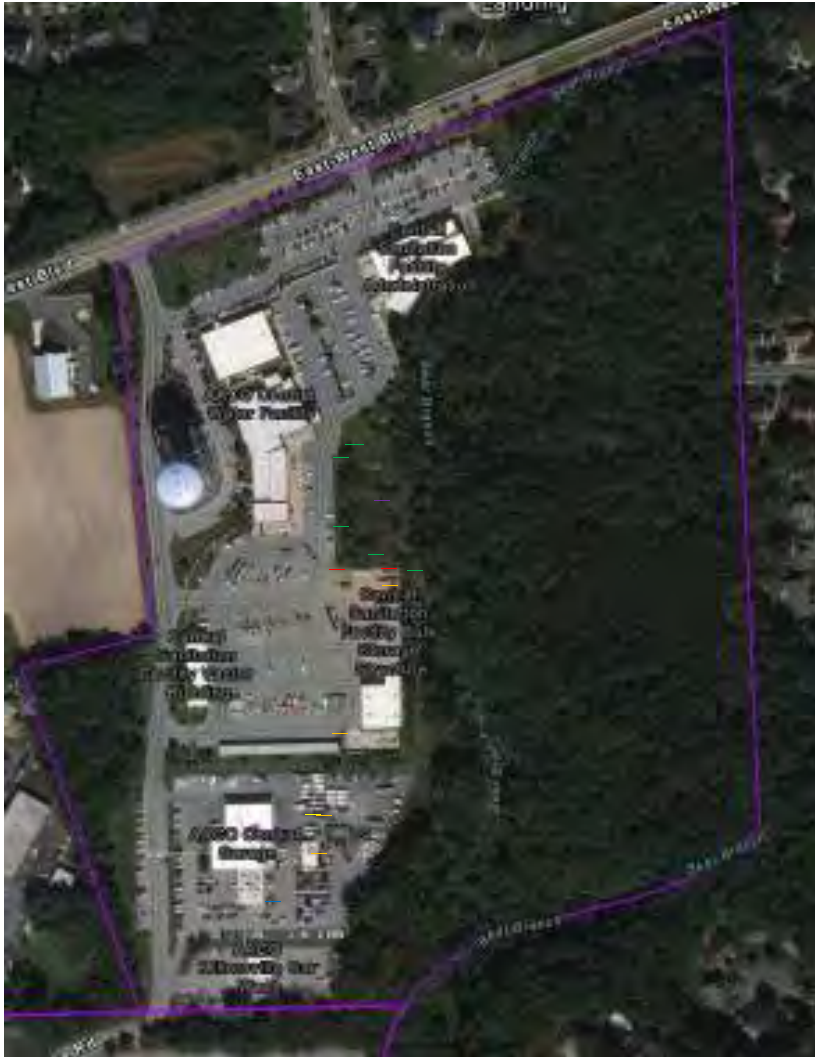
Figure 1: Aerial map of the Millersville Garage property Purple Outline = Parcel boundary Orange Point: Improper bulk solid storage Green Point: Inaccessible outfalls within detention facility Red Point: sedimented outfalls Blue Point: Washdown activity Yellow Point: Improper liquid storage Purple point: Detention Facility
