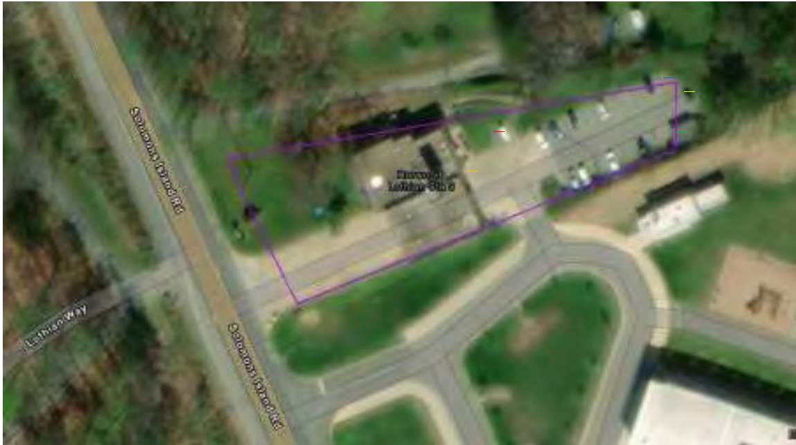
Figure 1: Aerial map of the Harwood Lothian Fire property Purple Outline: Parcel boundary Green Point: Storage shed Blue star: Outfall Red Point: fuel tank Purple point: improper bulk solid storage Blue point: curb cut draining parking lot Orange point: potential washdown activity Yellow Point: dumpster
