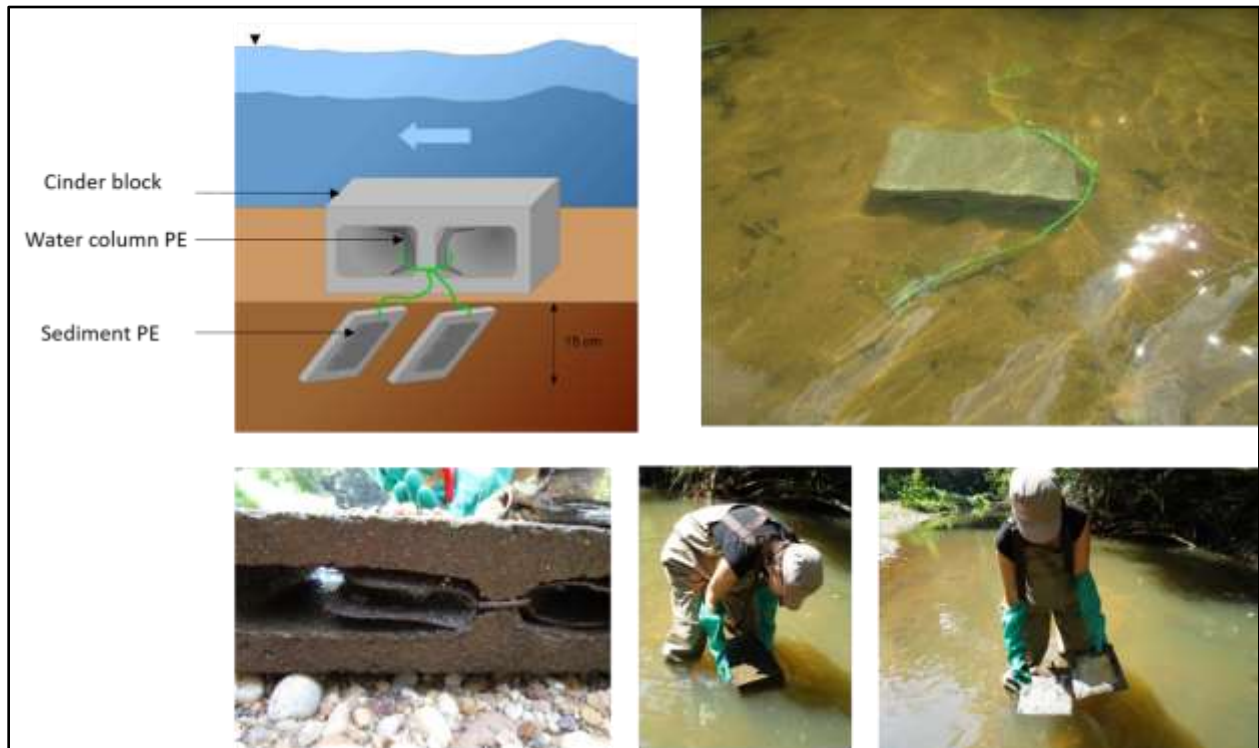
Figure 2: Passive sampler deployment in Anacostia River tributaries. Polyethylene (PE) sheets were enclosed in stainless steel mesh and were inserted inside a cinder block to measure water column concentration, or mounted into frames and inserted into sediments to measure sediment porewater concentration. Top left: a schematic representation of passive sampler deployment in situ. Top right: picture of passive sampler deployment in Anacostia tributaries. Bottom left: picture of water column PE inside cinder block. Bottom middle: cinder block containing water column PE is placed on the tributary bed, parallel to water flow. Bottom right: pictures of frames that are inserted into sediments to measure sediment porewater concentration.
