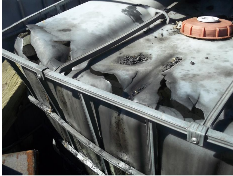
3/9/2023 Inspection – Cracked tote.
