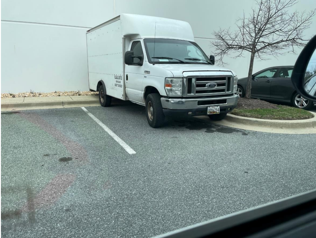
2/24/2023 Inspection – Dark staining under vehicle. Slight red stains indicate a potential transmission leak.
