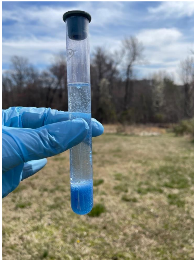
3/22/2023 Inspection – Detergents results from sampled manhole upstream of right pipe.
