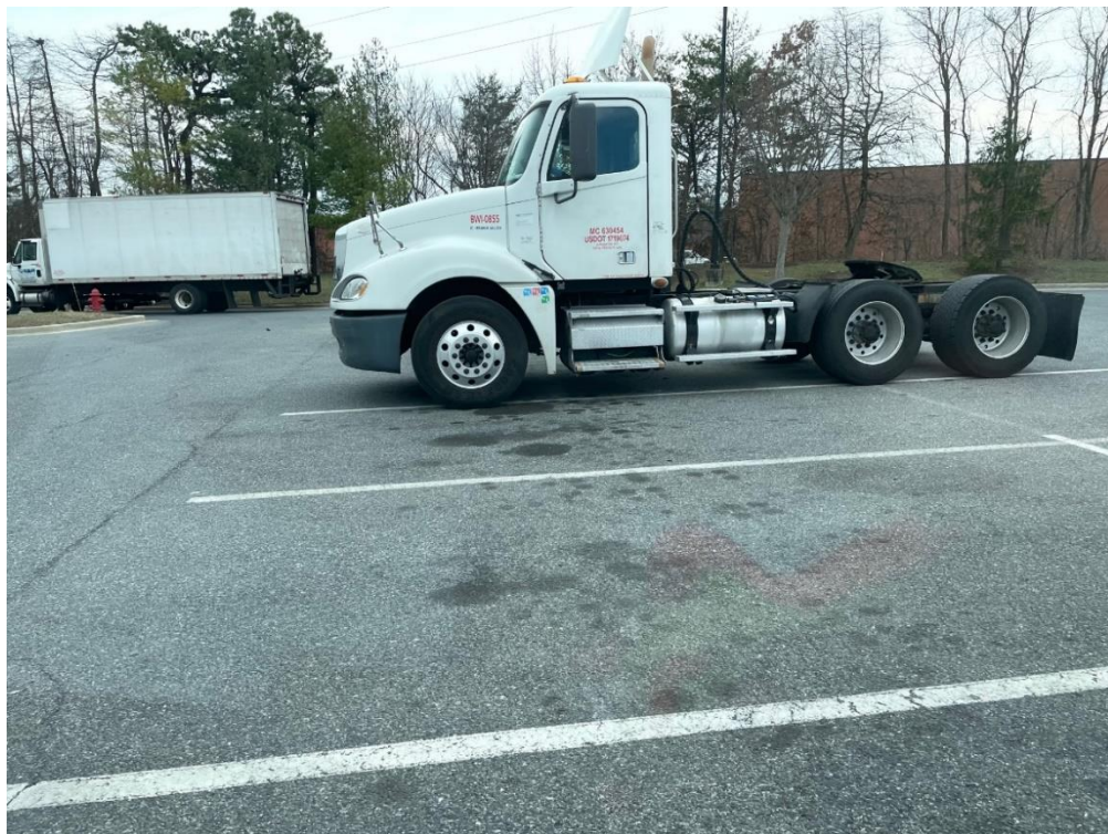
2/24/2023 Inspection – Stains under parked tractor. Slight red stains indicate a potential transmission leak.
