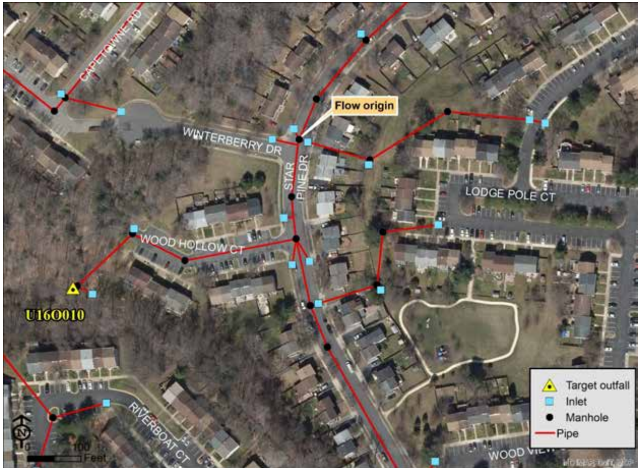
Figure 2. Area map, showing the location of the target outfall and associated infrastructure
