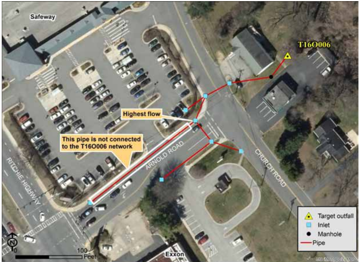
Figure 2. Area map, showing the location of the target outfall and flow patterns observed in the associated infrastructure on March 8, 2019
