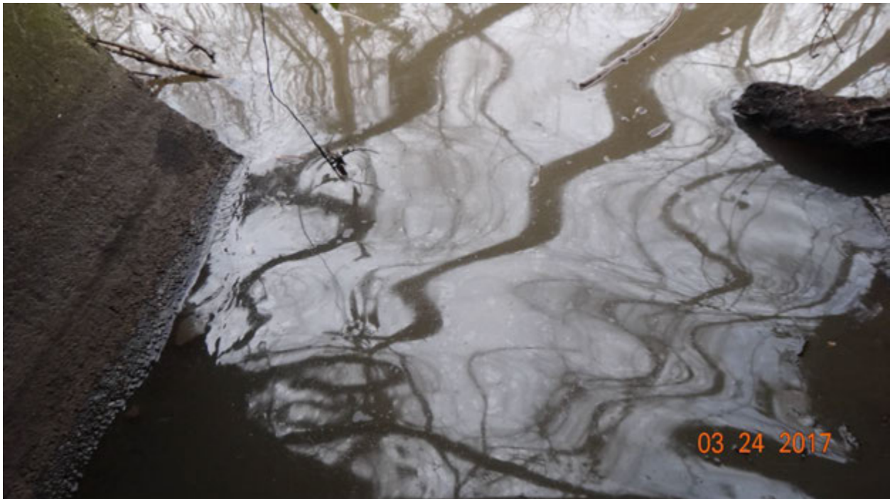
Figure 2. Evidence of oil on the surface of the discharge from the outfall on March 24
