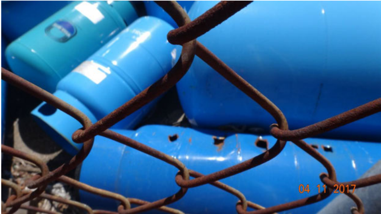
Figure 2. A detail view of one of the pressure tanks seen with rusting holes from previous punctures
