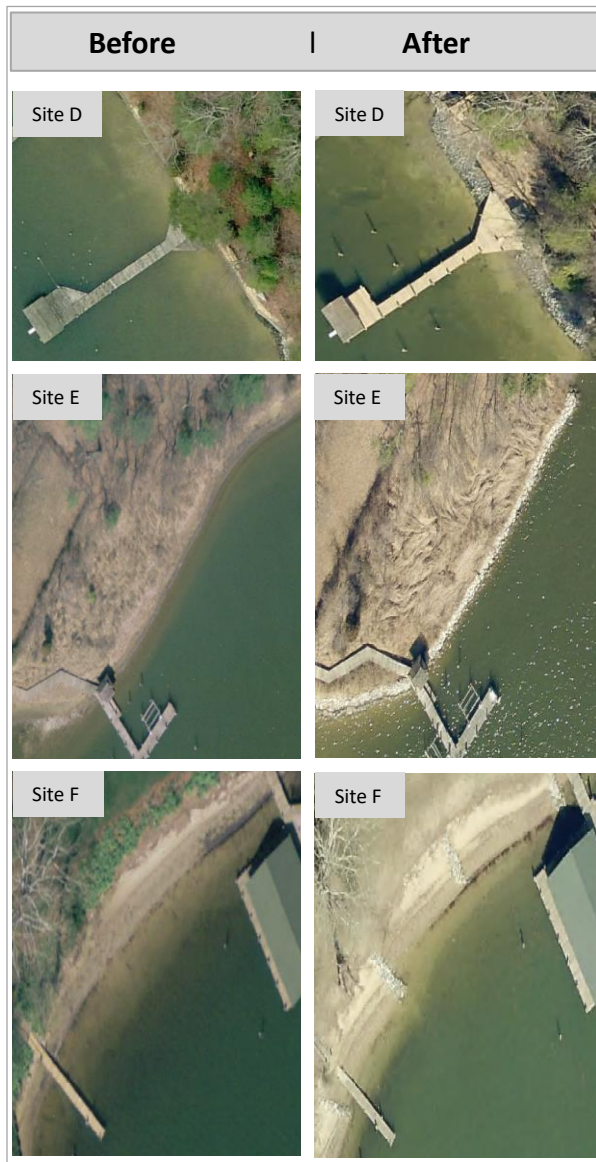
Figure 8. Shoreline Stabilization Site Examples
