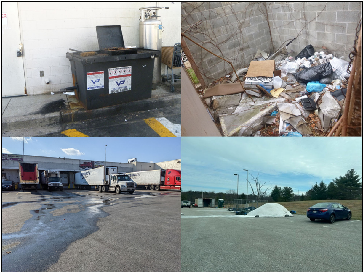
Figure 2. Examples of upland pollution sources. Clockwise from top-left: open kitchen waste grease container and staining of pavement, accumulation of trash in dumpster bay, evidence of improper commercial vehicle washing, and an uncovered pile of road salt.
