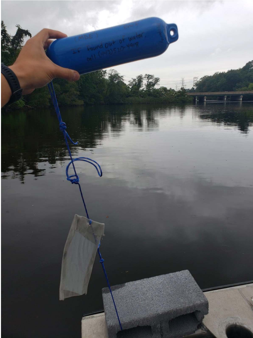
Figure 2: Passive sampler deployment. Polyethylene (PE) sheets were enclosed in stainless steel mesh and attached to a cinder block (picture) or to a green post.
