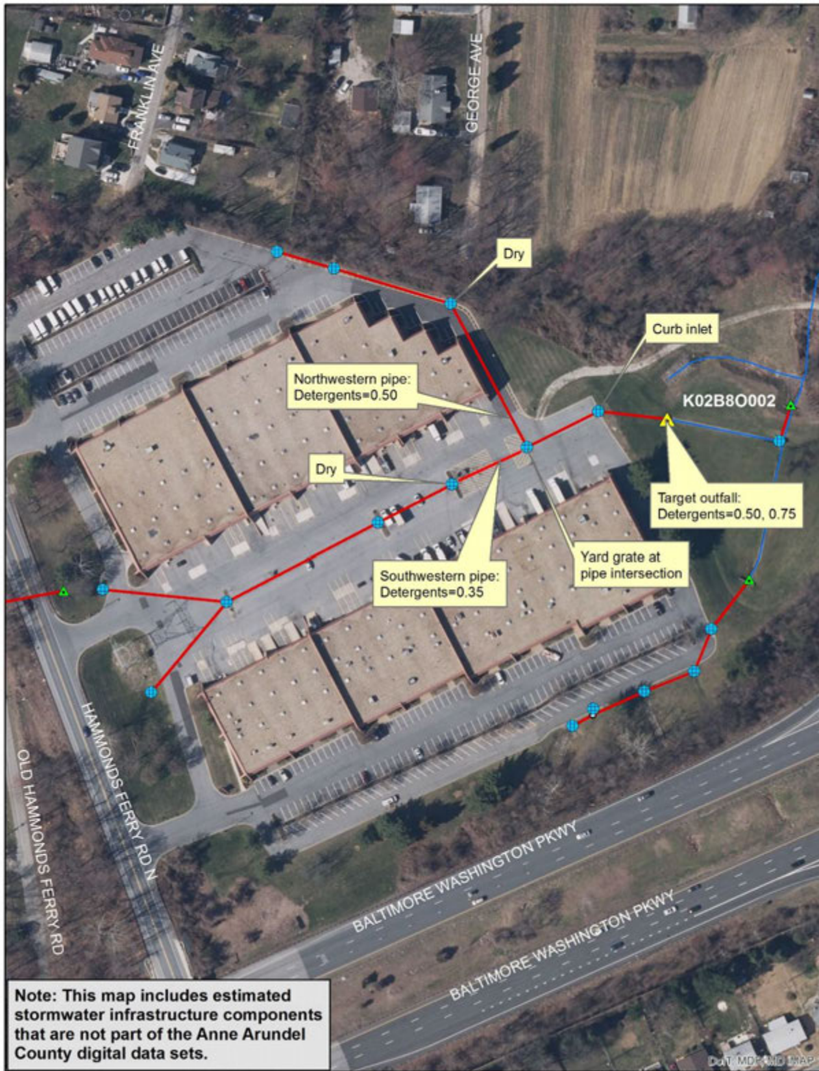
Figure 4. Area map, showing detergent concentration test results obtained during the outfall discharge testing and subsequent trackdown
