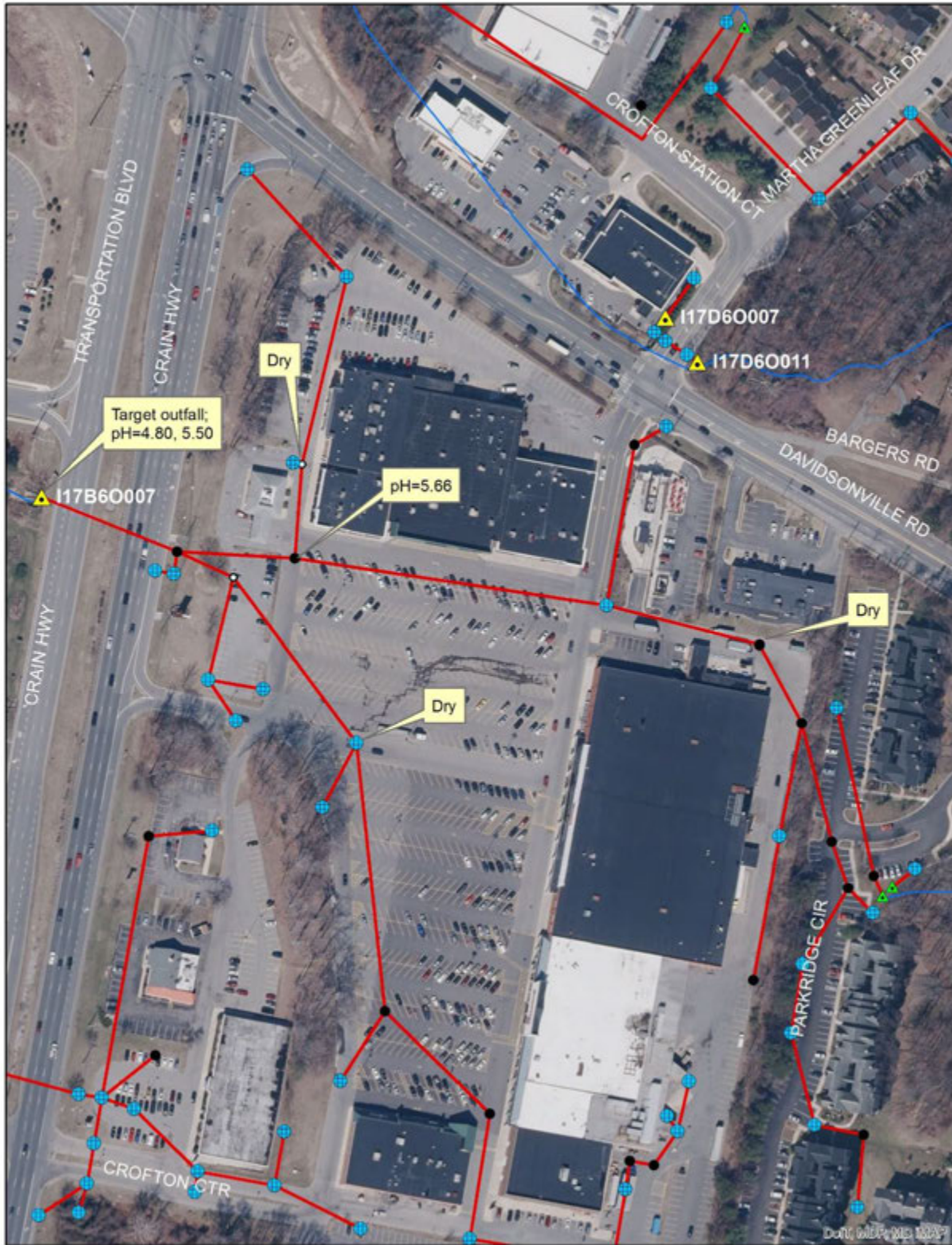
Figure 3. Area map showing results of trackdown efforts along pipes leading to the target outfall, I17B6O007
