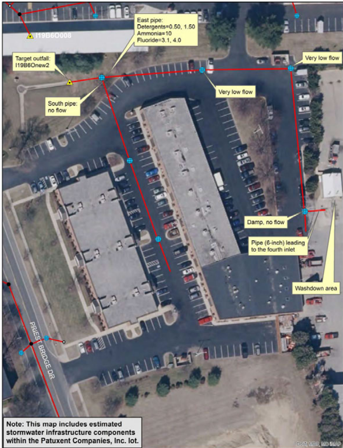
Figure 5. Area map, showing flow observations, and listing above-action-level readings for the water in the pipe from the east at the intersection
