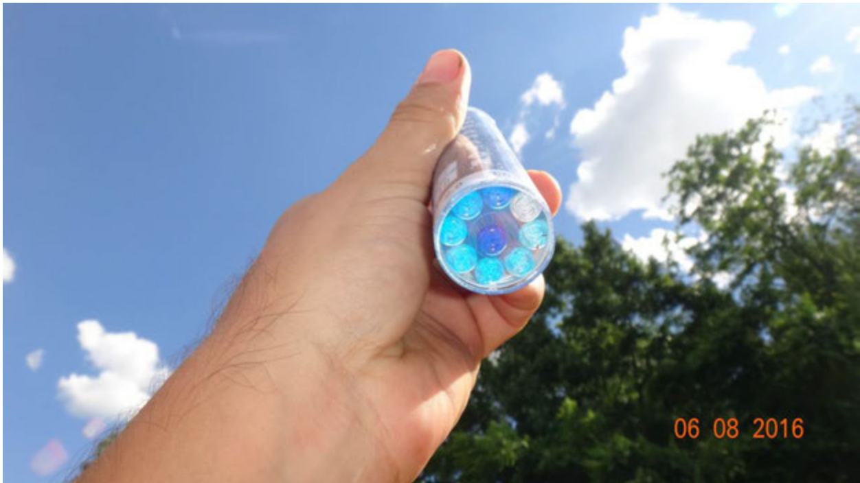
Figure 3. The test result (center) showing the color far exceeding the potential of the test to determine the extent of detergents in the sample; a sample with a detergent level of 3.0 mg/l would have a blue color that matches the color of the vial at top of the outer circle (darkest blue)
