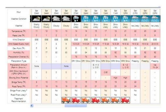
Figure 2. MDSS Hourly Weather Forecast With Treatment Recommendations
