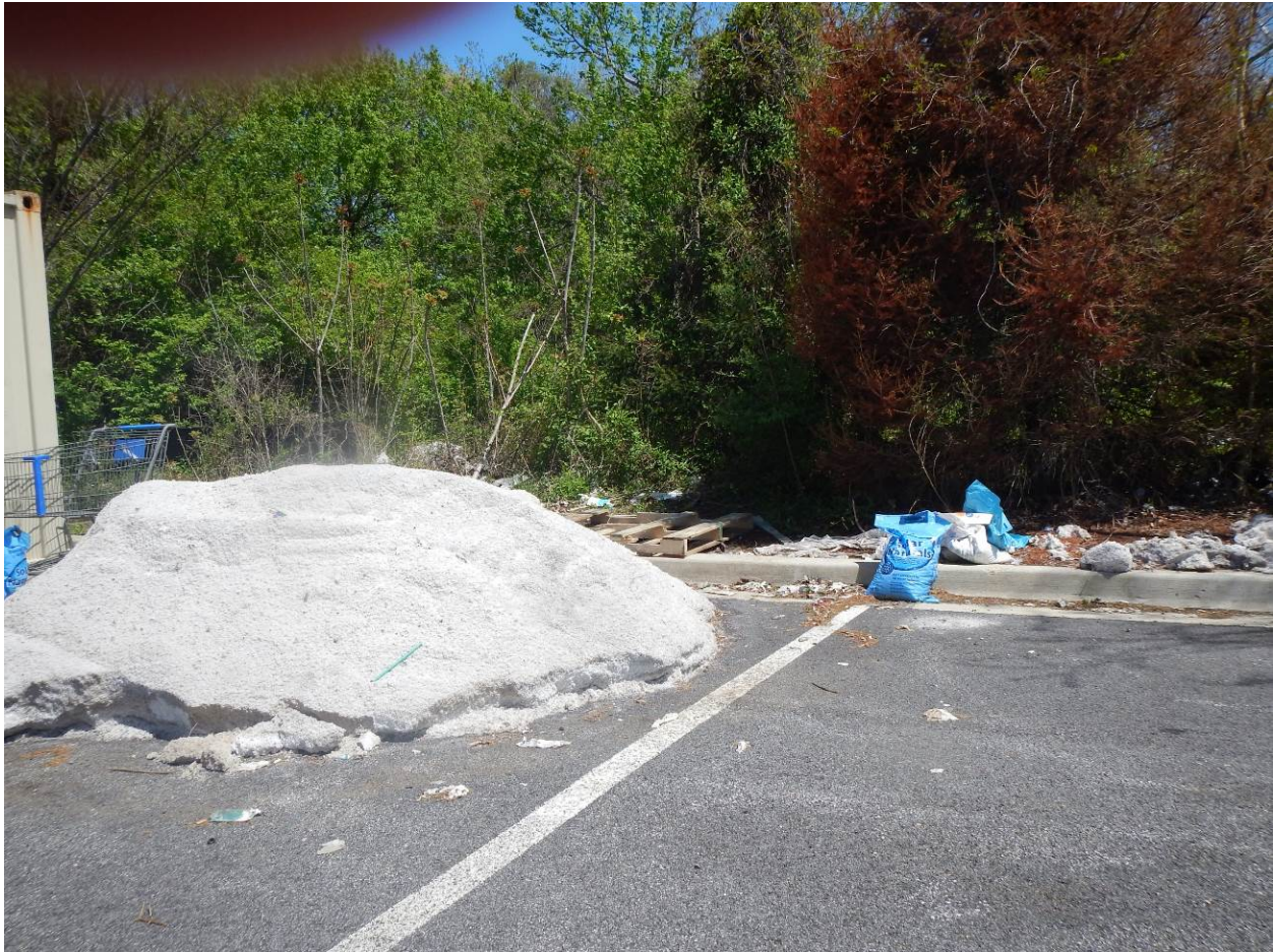
Figure 1. A large, uncovered pile of road de-icing salt in the parking lot, small piles of road salt on the ground, and several bags of water softener salt crystals found on the day of the site visit
