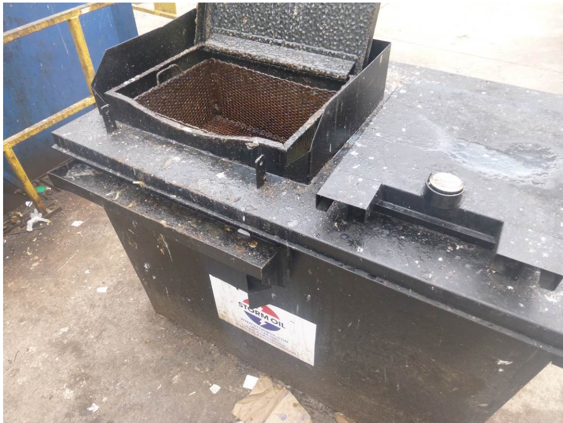
Figure 1. Cooking oil collection container found with an open lid; the container was located uphill of a curb inlet in the same parking lot
